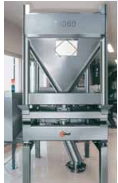
Container discharging station above a tablet press
