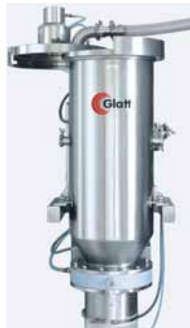
Separator of a PCS-PRO with swiveling lid for an easy filter exchange
