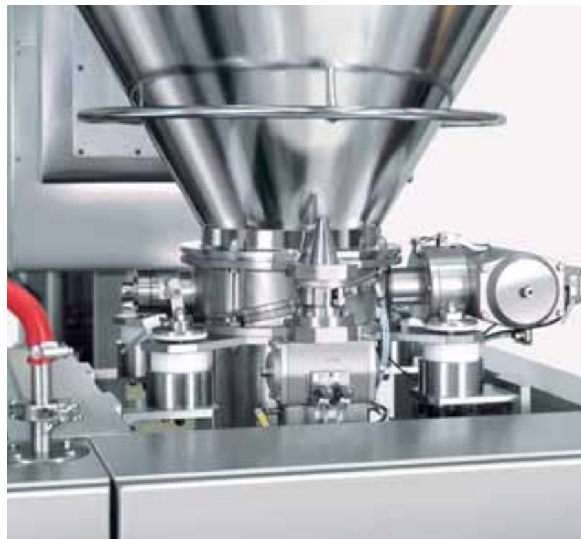
IBC discharge using the Glatt SKS isolation valve system
