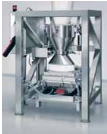
Vibration dosing sieve, integrated in a discharge station for big bags (supersacks)
