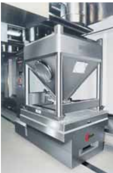
AGV for automatic weighing and charging of IBCs
