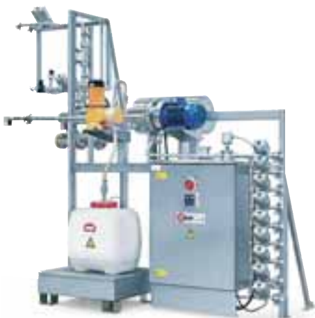
CIP rack for preparation of washing recipes
