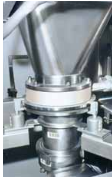
Docking system using an inflatable axial seal, after docking
