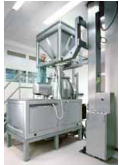
L 1500 lifting device for discharging containers into a VG 600 vertical granulator
