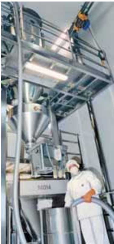
Discharge station, docking under the FBE with bottom discharging
