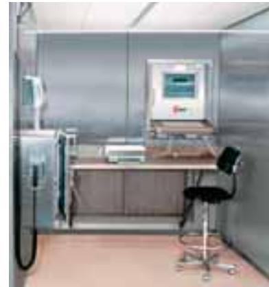
Weighing cabin for small components
