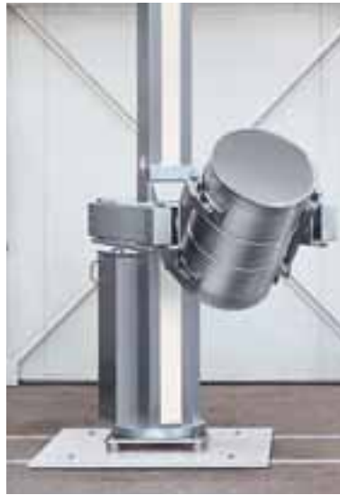
Drum discharging in longitudinal direction using EL 600 stationary lifting device
