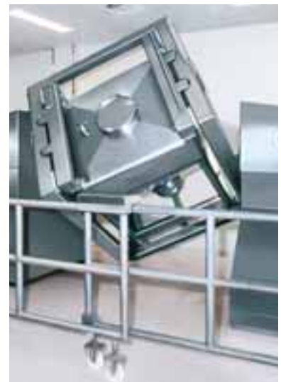
CMK 1000 special design, mixing between two columns
